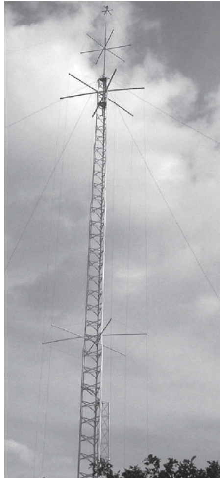
Figure 21 — The pickup antenna was this 80 foot caged, folded monopole for the Texas measurements.
