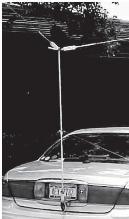
Figure 1 — Typical mobile antenna with multiple resonators .
