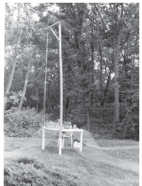
Figure 8 — Late '80s tests with chicken wire fencing for a ground plane
